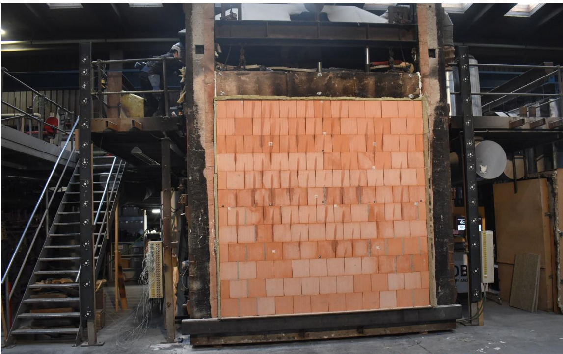
Photo No. 20 240 minutes in the test. Test stopped
