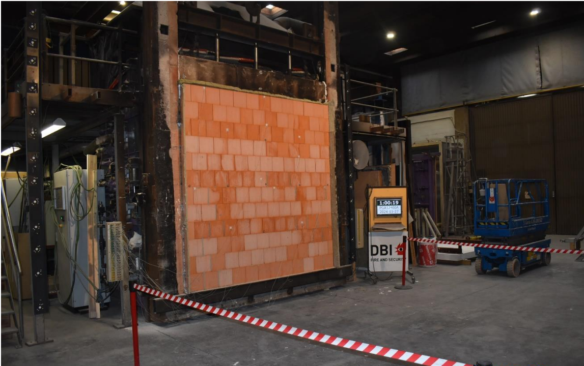
Photo No. 15 60 minutes in the test, with no visible changes
