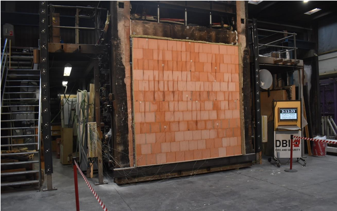
Photo No. 19 192 minutes in the test, with no visible changes
