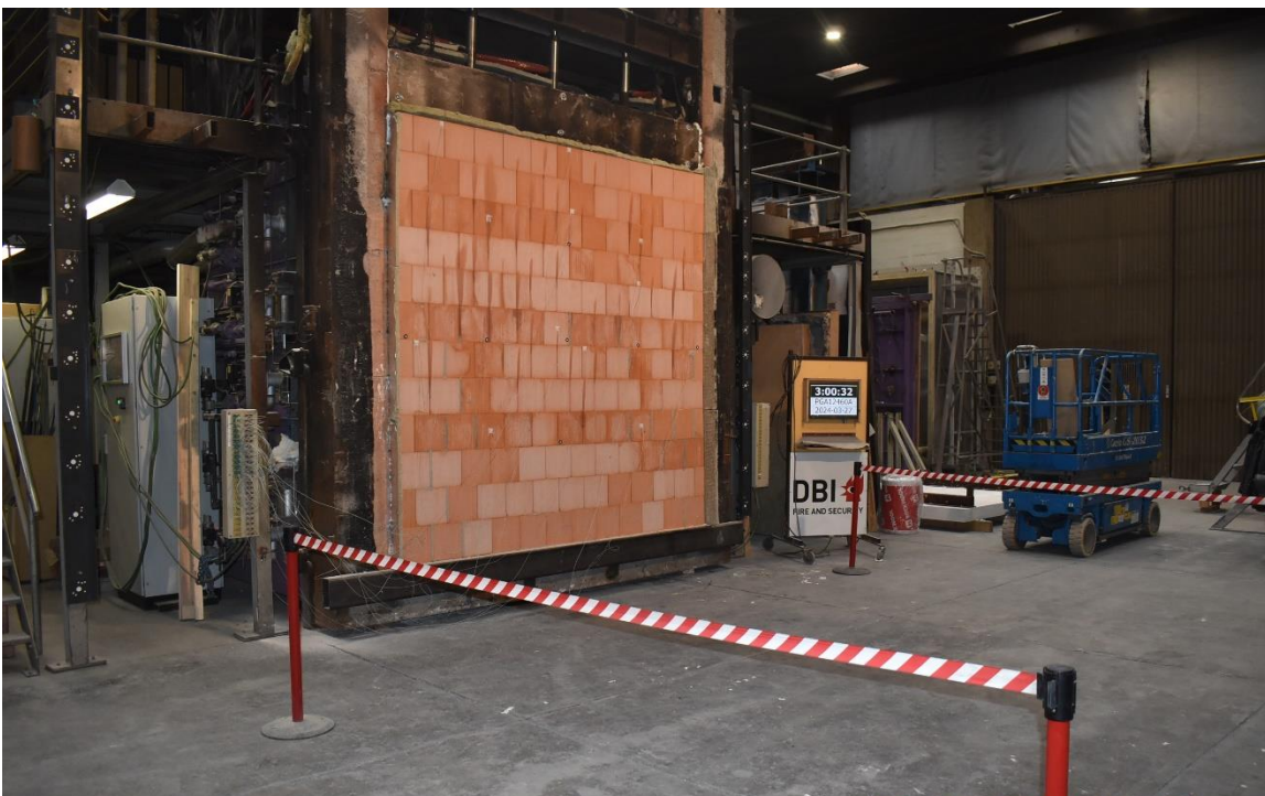
Photo No. 18 180 minutes in the test, with no visible changes
