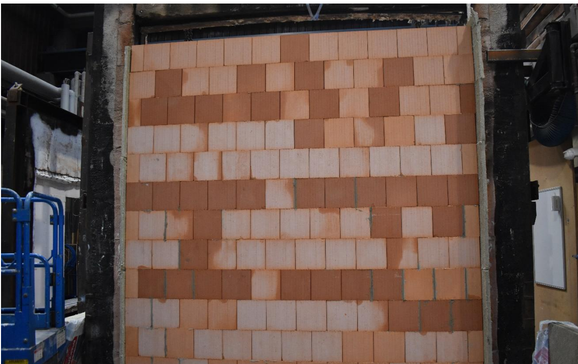
Photo No. 10 Build up with the last finish of mortar put in between the joints
