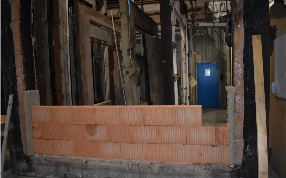
Photo No. 3 Three layers of the wall mounted to the bottom.
