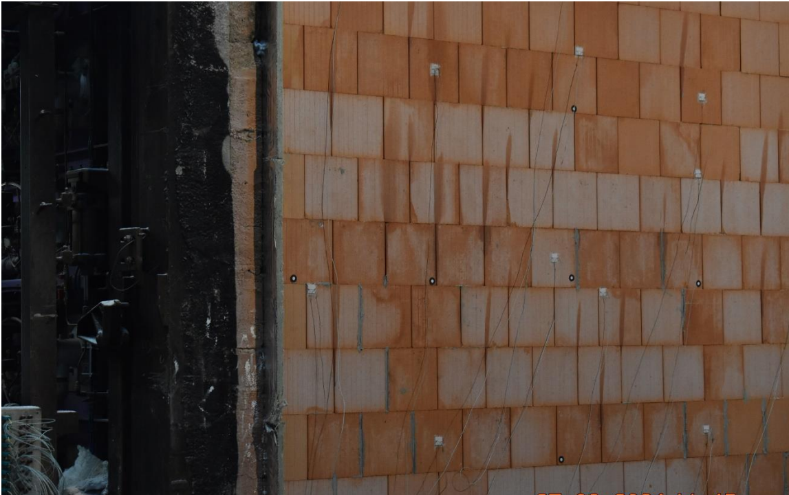
Photo No. 17 163 minutes in the test, with visible moisture from the joints
