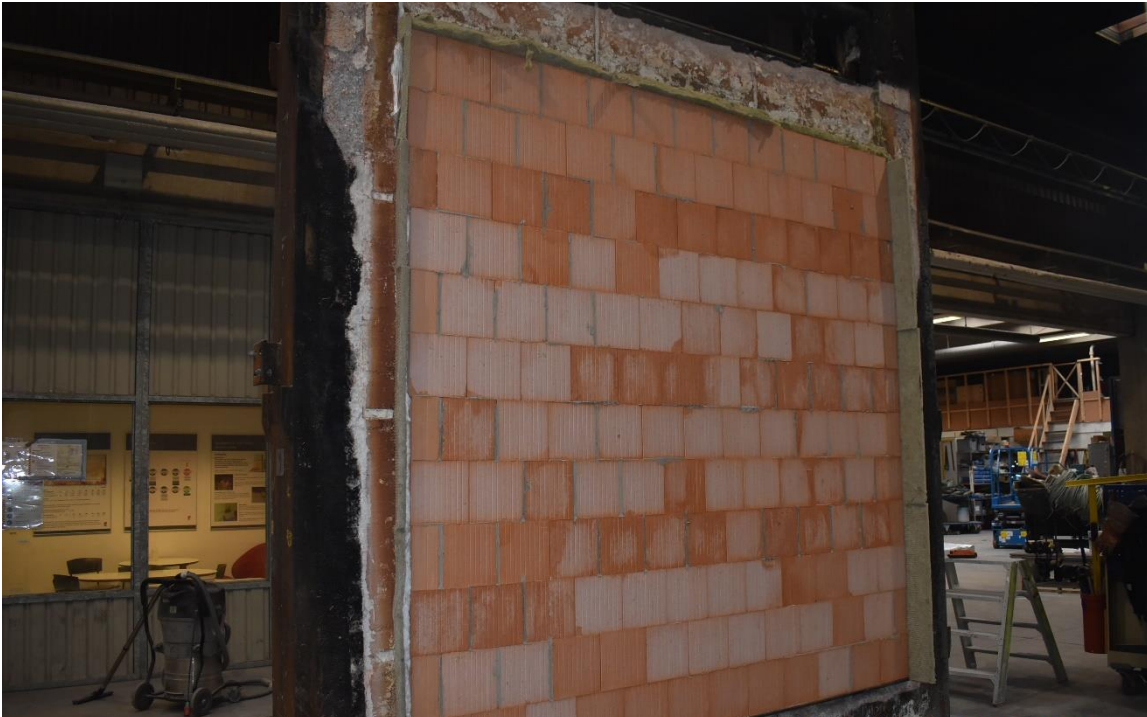
Photo No. 11 Wall finished and ready for thermocouples
